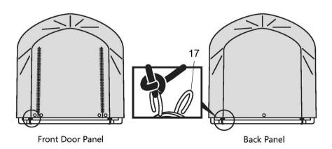
7. Tie the other side of the roof cover rope end on parts 17 (Fig A) and then through the door panel eyelet and tighten again. (Fig B)
