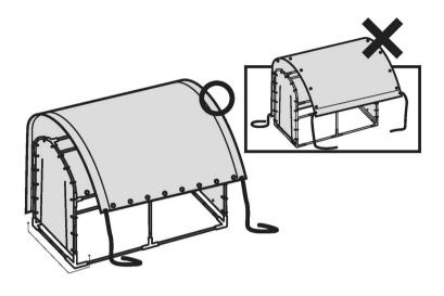
6. Tie one side of the roof cover rope ends on couplers (17).
